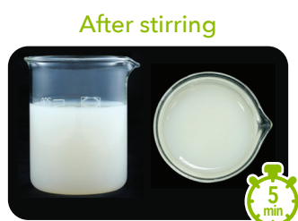
Figure 2: Uniform suspension of DVP 30-WD in water
