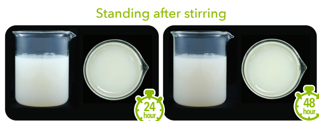
Figure 3: DVP 30-WD in suspension over 48 hours
